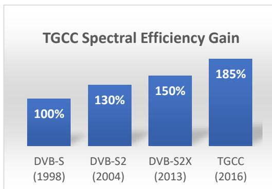
Fig. 2: TGCC Spectral Efficiency gain in Satellite Communication
