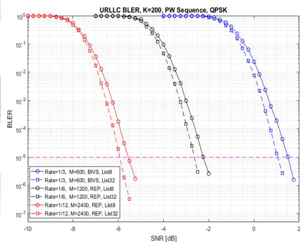
Fig. 4: Tsofun 5G implementation gain (0.5dB without adding complexity)
