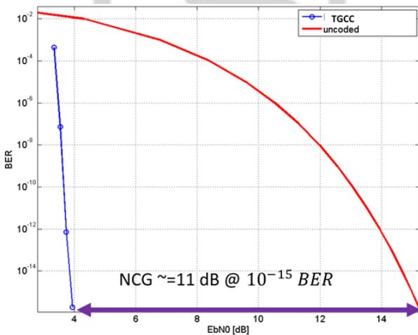
Fig. 3: TGCC Net Coding Gain in Fast Optical Networks
