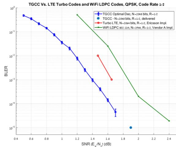
Fig. 1: TGCC advantage over Turbo (4G/LTE) and LDPC (802.11ac Wi-Fi) codes
